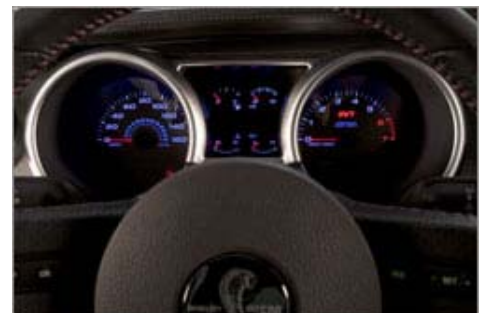
The unique gauge cluster places the tachometer in the dominant position, along with a new supercharger-boost gauge and titanium finish.
