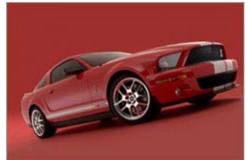
Shelby Cobra GT500's LeMans and tri-bar stripes inspired by classic Shelby designs, functional front splitter and air extractors inspired by aerodynamics of the 2005 Ford GT.
