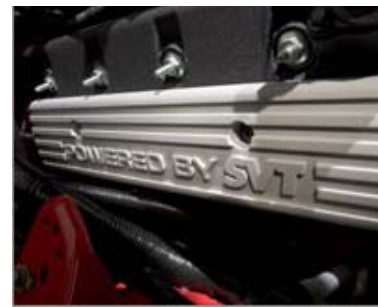
Cast "Powered by SVT" coil covers for four-valve heads sourced from Ford
